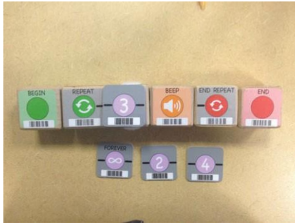
Figure 2. Repeat loops program. Note. The program above shows a syntactically correct repeat loops program using the number 3 parameter. This program will tell the robot to beep three times. Pictured below the program are choices of other number parameters that can be used for this type of program.
