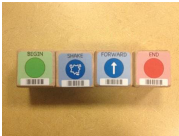
Figure 3. Basic program starting with Begin block and finishing with End block.
